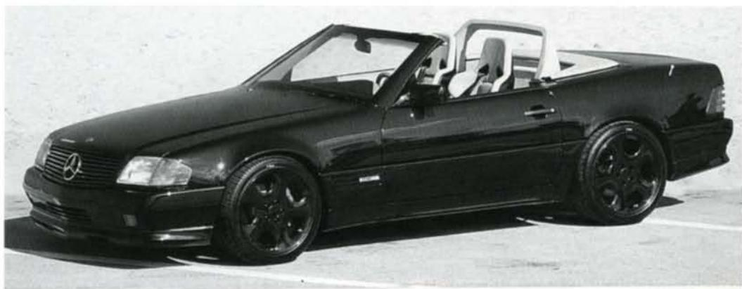
The modification includes sway bars, front and rear, by RENNtech; stiffer springs built to RENNtech specifications by Hyperco Springs; externally adjustable shocks made exclusively for RENNtech by Koni, and a rear sub-frame modification by RENNtech. The latter modification replaces the rear suspension pieces with aircraft grade adjustable links, allowing for better handling and more stable acceleration.
