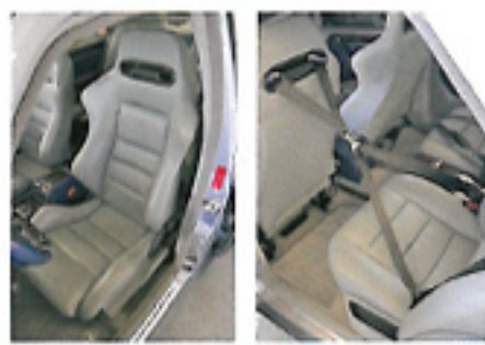
Retrofit, form-fitting Recaro seats connect with race-derived, complex Schroth harnesses.
