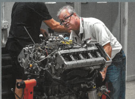
△ Hartmut hard at work fettling a 6.0-litre M117 V8 AMG engine.
